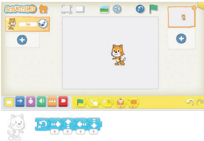
Figure 1.6 Scratch Jr programming for drawing a square
